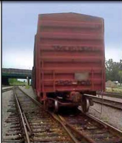
*Parking a rail car too near a switch causes clearance problems for trains passing on the adjoining track.*
