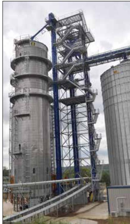
*Closeup view of the facility's 7,000-bph Zimmerman grain dryer, 20,000-bph InterSystems receiving leg, and four-hole InterSystems distributor.*
